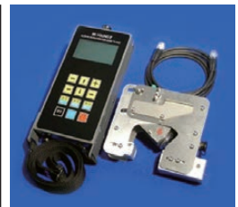
Modified cable insertion measurement equipment
