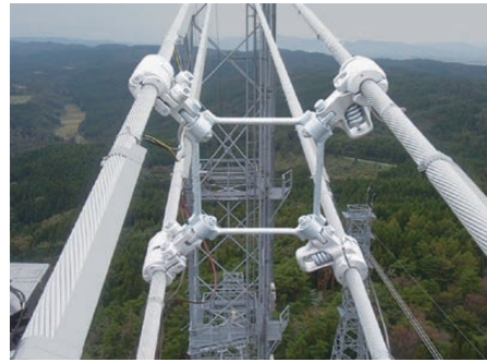
Simulation of snow accretion with 4 conductor loose spacer during the test
